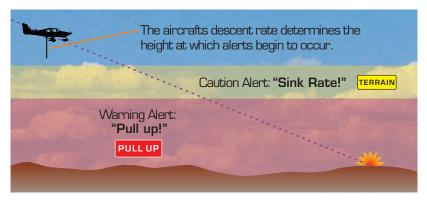
Figure 2-38: Excessive Descent Rate Alert Condition
