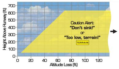
Figure 2-42: Altitude Loss After Takeoff Graph
