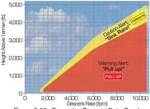
Figure 2-39: Excessive Descent Rate Graph
