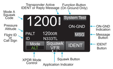
Figure 2-5 Transponder Application Screen
