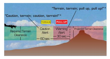
Figure 2-35: Reduced RTC Alert Condition
