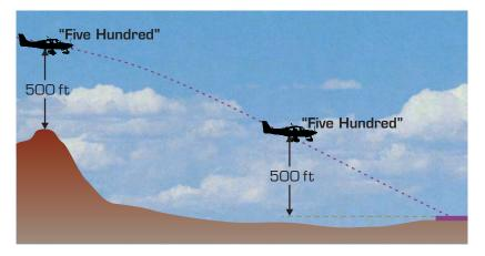
Figure 2-43: Altitude of 500 Feet Callout Condition
