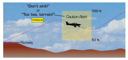
Figure 2-40: Negative Climb Rate or Altitude Loss After Takeoff Alert Condition
