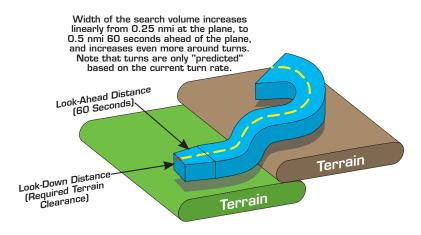
Figure 2-33: Forward Looking Terrain Avoidance (FLTA)
